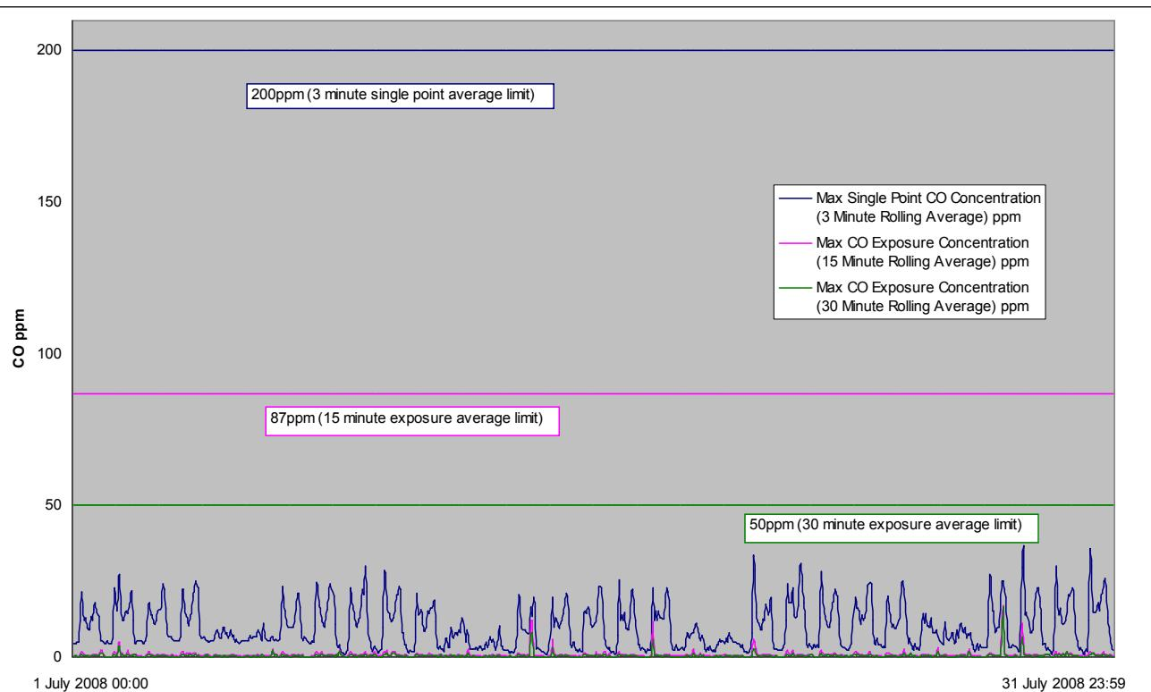
**Figure 1: Graph of CO Exposure and Single Point Averages for July 2008**
